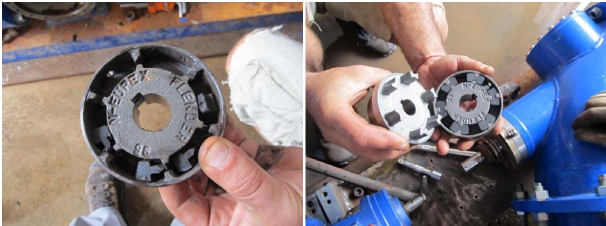
Fig. 11 - Coupling joint damaged on left and the new one on right.
